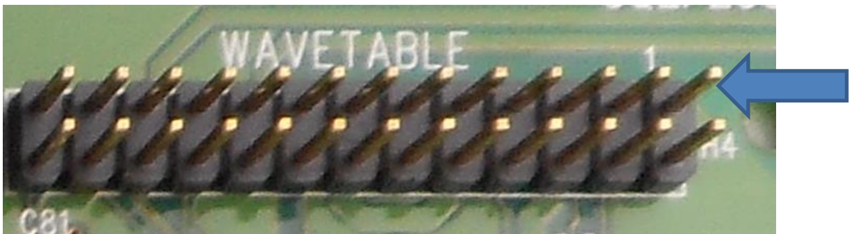
Figure 6 - Marking for pin 1
