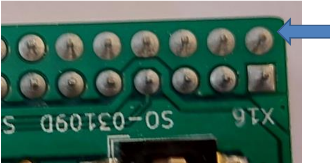
Figure 5 – X16 pin 1 and 2 location
