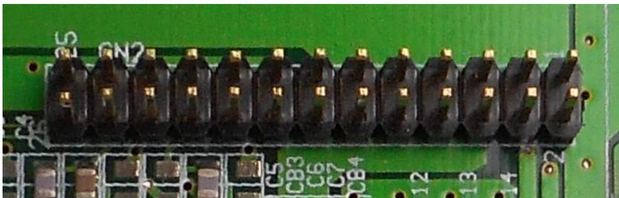
Figure 8 - Marking for pin 1 and 2
