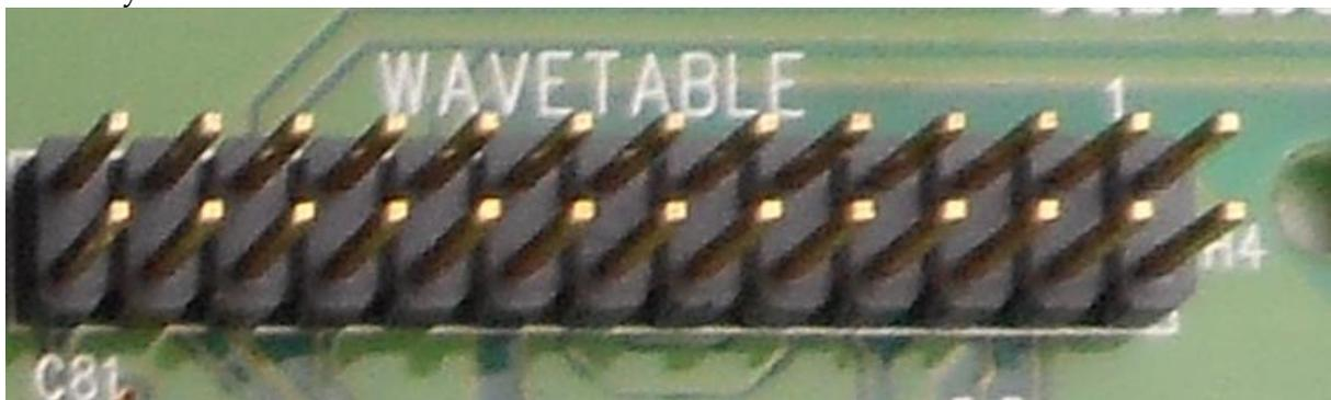
Figure 7 - Marking for pin 1
